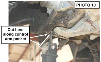
24. While supporting the differential, remove the upper driver side bolt and remove the two nuts with a 21mm wrench on the passenger side that secure the differential to the frame. Retain the two passenger side nuts as they will be re-used. Also remove the factory bump-stop using a 15mm wrench, retain for reuse.
