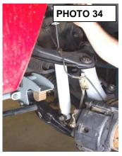
50. Install the wheels and tires. Lower to the ground and tighten the lower control arms bolts with a 18mm & 24mm wrench. Tighten the kicker bars at this time with a 21mm & 22mm wrench.
